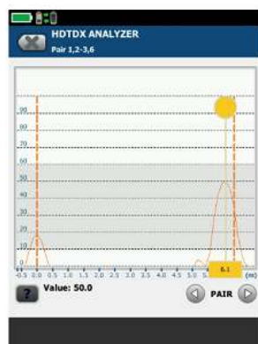
High Definition Time Domain Cross talk (HTDX) shows the far end connection is clearly the issue
